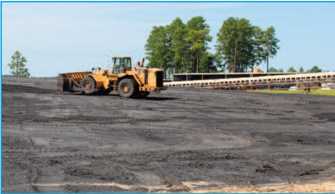
A 25-day supply of coal is maintained at the R.D. Morrow, Sr. Generating Station to ensure adequate onsite fuel supply for the plant's two units.
